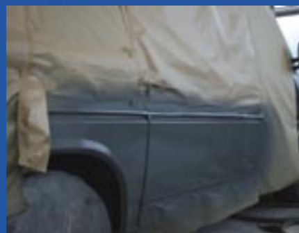
6. Application of sprayable filler or putty
