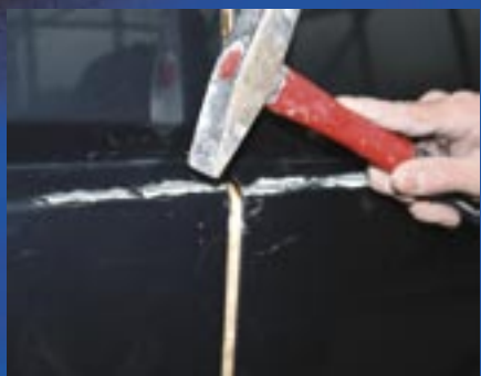
2. Coarse treatment of the defect
