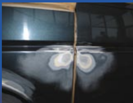
3. Sanding the defect
